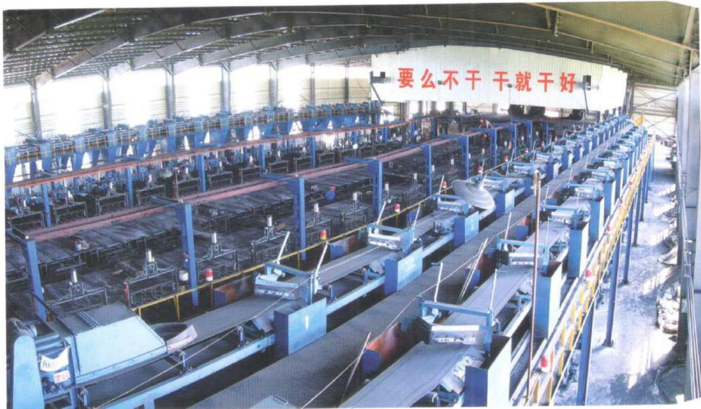
造型自动生产线 Automatic molding production line
